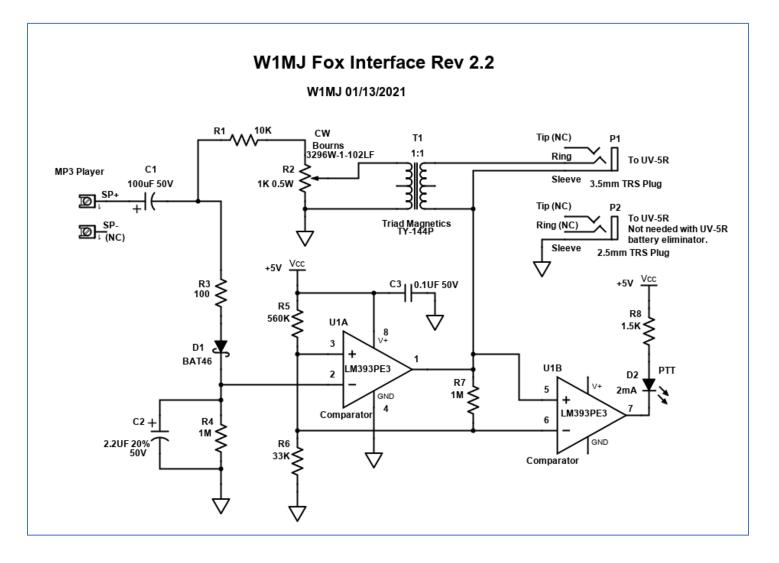
Audio peaks from the MP3 player charge capacitor C2. R3 limits the loading on the player to prevent distortion. When the voltage on C2 exceeds the reference voltage at U1-3, comparator output U1-1 pulls the radio PTT line (P1-Sleeve) to GND to key the transmitter. Hysteresis is provided by R7 to ensure clean PTT switching. When the audio pauses, C2 discharges through R4, ending transmission after approximately 2 seconds. LED D2 indicates that PTT is active.
