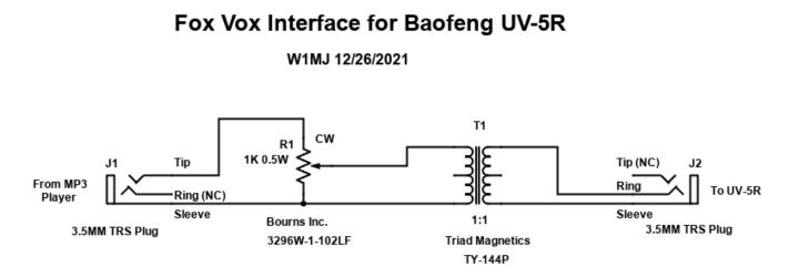
To avoid the need for the strong sub-audible tone, the circuit shown below is used. It is intended to be a better VOX. It keys the UV-5R PTT. The PTT return via the battery eliminator GND appears to suffice, but J3 is shown in the diagram just in case.
